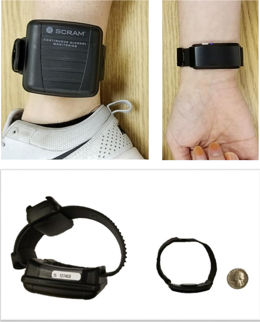
Figure 1. AMS SCRAM ankle bracelet (left) and BACtrack Skyn wrist monitor (right) displayed side-by side. The top panel displays these devices as worn on ankle/wrist, whereas the bottom panel displays them to scale. The approximate weight of the devices is 6oz (SCRAM) and 1oz (Skyn prototype), respectively.
