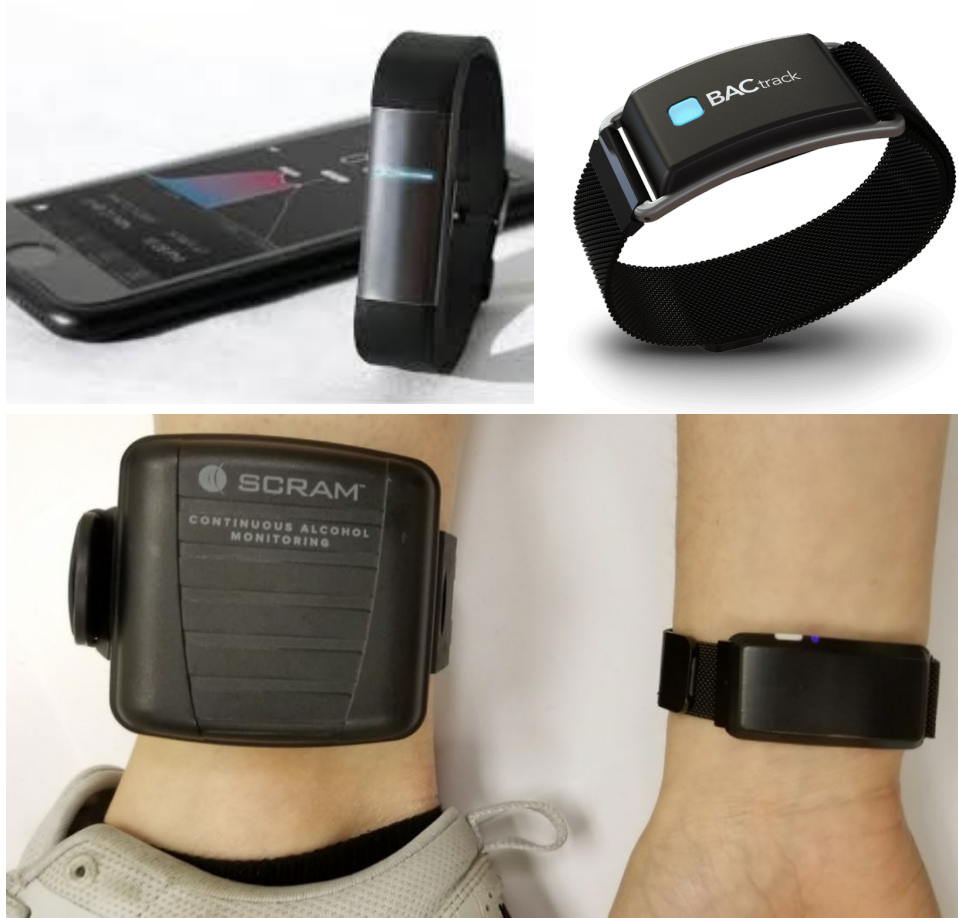
Figure 1. Top panel displays two new generation transdermal wrist sensors—Milo (left) and BACtrack (right). Bottom panel displays old-generation (AMS SCRAM; left) and new-generation (BACtrack Skyn prototype; right) devices to scale, side by side. Bottom panel adapted from (10).
